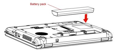
Figure 6-3 Installing the battery pack
